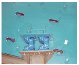
AB-D suspension of a dewatering screen
