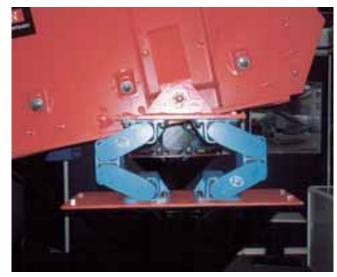
AB suspension of a circular gravel screen
