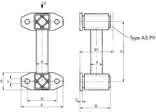
Type AS-PV with one offset flange
