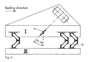
rotate and are joined absolutely rigid, so that they synchronize at once when switched on, setting-up linear oscillations.
