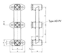
Type AD-PV with offset flanges
