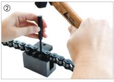
The fork (A 1) is placed through the chain at the outer link which is to be removed. The fork is then supported by the anvil and the bearing pins are driven through the chain using punch (B) 2. Multiple strand chains can also be broken in this way, the fork should then be placed in the top strand of the chain.
