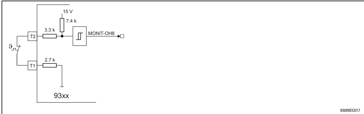
Input circuit for the connection of the measuring sensor
